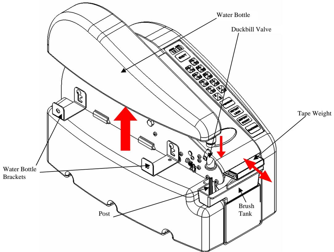
**Figure 4 – Filling the Water Bottle, Adjusting the Brush Tank Water Level, Adjusting the Tape Weight**
