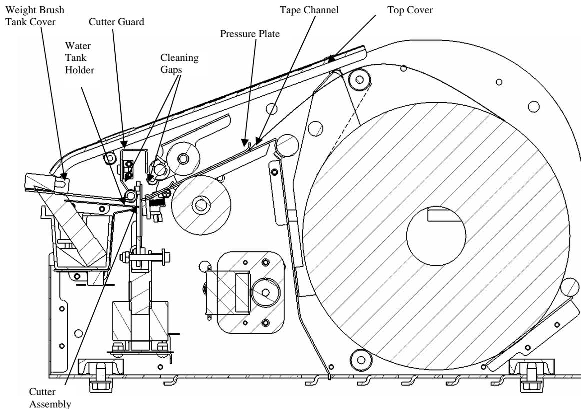
**Figure 9 – Cleaning the Cutter Assembly, Cleaning the Tape Path**
